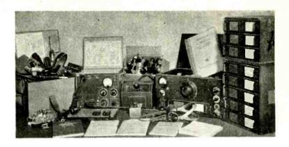
Equipment issued to Reservists for use at home includes a 30-watt portable h.f. transmitter (Type 5G) and a communication-type receiver.
