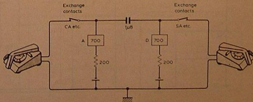
Fig. 2 (over page). Complete circuit diagram of the exchange. Resistors of 200Ω in series with A and D relays are 1W; 100Ω resistors across B and C relays are ½W; all rest are ¼ types.
