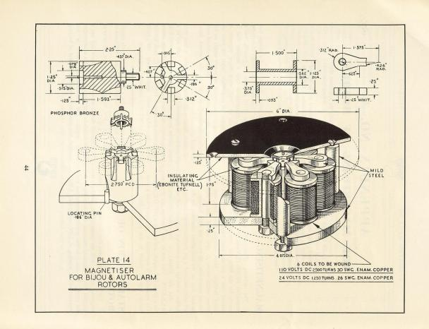
the stabilising strength constant. Experiment will be necessary to obtain that setting of the variable resistance which gives correct stabilising figure strength. In use, place the magnetised rotor into the stator, set the variable resistance at a high value, depress switch momentarily,
