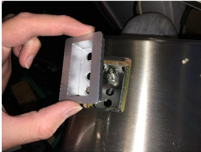
Once the escutcheon is out of the way, there is another nut on the antenna connector, remove this and the connector is then free from the back cover.
