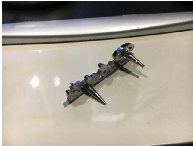
There are 4 rubber feet under the radio, which will simply pull off. It may be necessary to pry them with something thin and metallic, so as not to separate the rubber from the pin.
