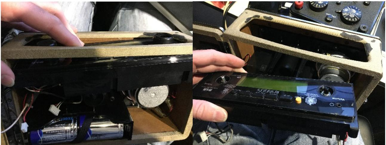
Now you can begin to remove the battery box/ speaker baffle. This is very fiddly! There are 5 plastic nuts (actually, a plastic thing with a metal insert...), 2 along the top, one under the speaker, and 2 in the battery box. They all need to be removed.
