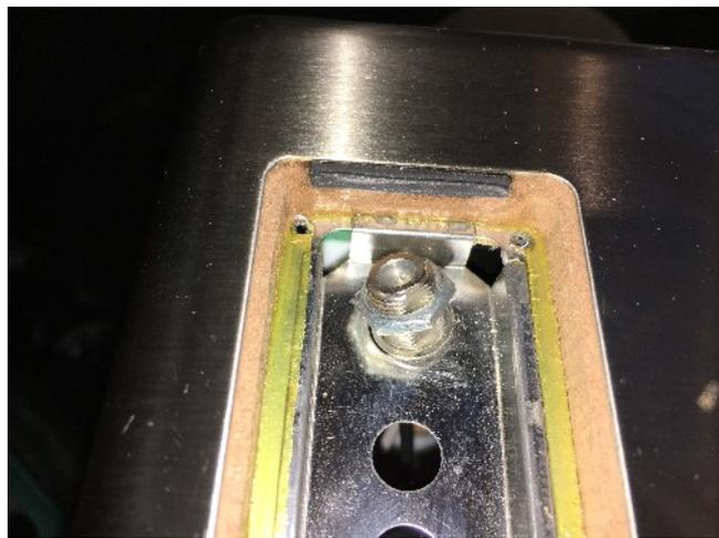
With the back cover open, you should see the back of the speaker, the 2 leads connected to it can be removed by gripping the connector and gently pulling it.
