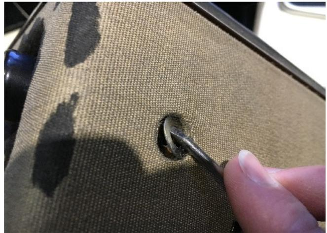
Once these are out you can begin to extract the chassis, firstly though, remove the control knobs from the radio, they just pull off.
