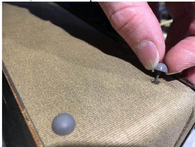
That's it! You should now be left with an empty radio case. Only things left to do now are to unscrew the hinge, and carefully pry off the clasp that holds the case shut. Save all your fixings in a bag or something for later when you re-assemble the radio. Everything should be re-fitted to the case in the reverse order, all plugs that were unplugged previously only fit into their own sockets that they came out of.
