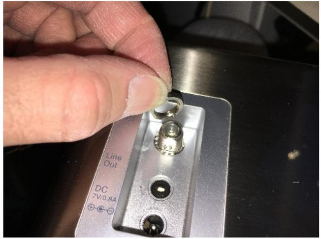
Open the back, locate the black box which contains the antenna connector, and the line out DC in sockets, pull out the 2 plugs, one for the battery box and one for the audio. Do not pull the antenna cable, or the thick black cable, as these are permanently connected.
