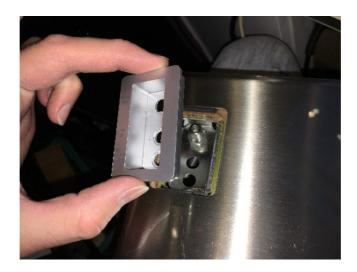
Once the escutcheon is out of the way, there is another nut on the antenna connector, remove this and the connector is then free from the back cover.
