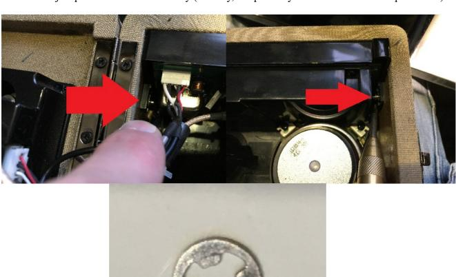
Once the handle is off, this will expose the threaded bushes (big bolts with holes in them?!) which hold the radio chassis in the case. Unscrew these with a large screwdriver, taking care not to damage them.
