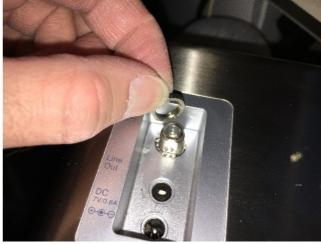
Open the back, locate the black box which contains the antenna connector, and the line out DC in sockets, pull out the 2 plugs, one for the battery box and one for the audio. Do not pull the antenna cable, or the thick black cable, as these are permanently connected.
