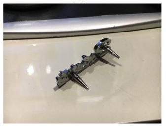
There are 4 rubber feet under the radio, which will simply pull off. It may be necessary to pry them with something thin and metallic, so as not to separate the rubber from the pin.
