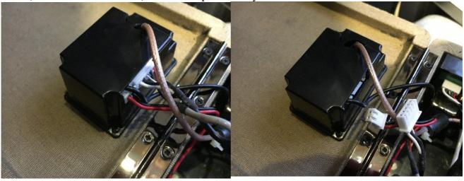
Remove the 4 screws in the corners. This will release the box and the plastic escutcheon from the back. The escutcheon may need a gentle shove from the inside to get it loose!
