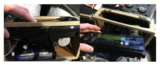
Now you can begin to remove the battery box/ speaker baffle. This is very fiddly! There are 5 plastic nuts (actually, a plastic thing with a metal insert...), 2 along the top, one under the speaker,
