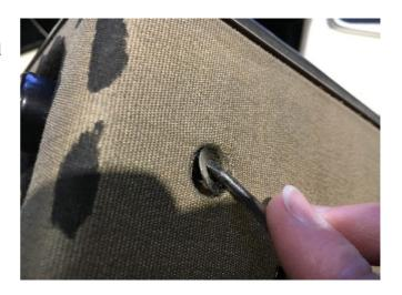
Once these are out you can begin to extract the chassis, firstly though, remove the control knobs from the radio, they just pull off.
