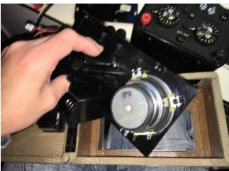
The 2 in the battery box are the most fiddly. Once these are removed, the whole assembly will just lift out of the case, the speaker mesh should also come out attached to the front with glue, but the glue may have dried out, in which case the mesh will still be in the radio.
