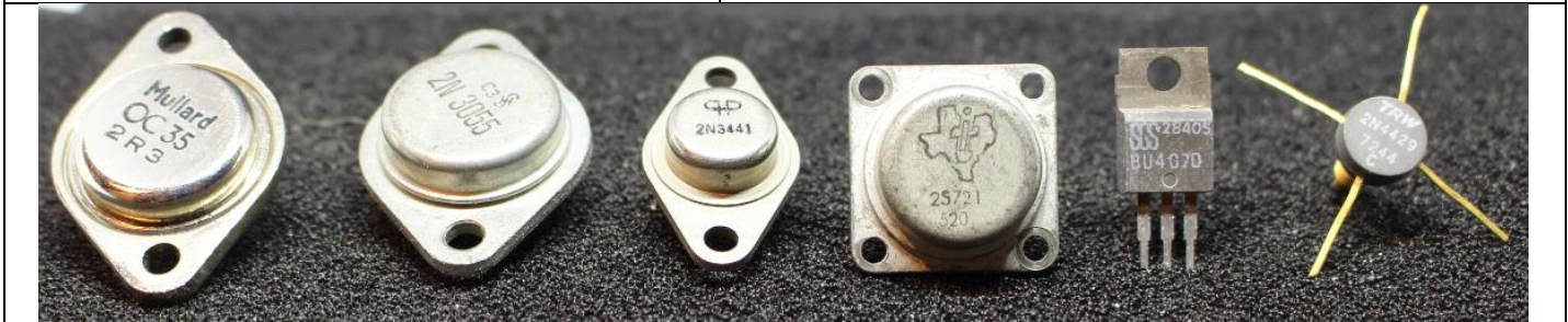
Figure 9 - Germanium and Silicon Power Transistors Left to right – OC35, 2N3055, 2N3441, 25721, BU407D, 2N4429
