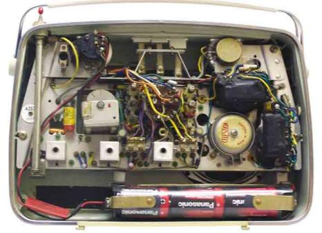
made use of the recently available Mullard AF11x series of alloy-diffusion transistors which offered improved HF performance over the earlier OC-series. The colour scheme for the set was new too, the case being light cream or ivory in colour with a tan rexine band around the middle. The metal trim is chrome and a telescopic aerial was provided for VHF reception, capped by a translucent red plastic 'pip'.
