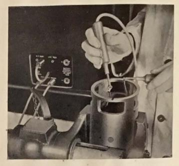
Fig. 13. Testing field coils for continuity.
