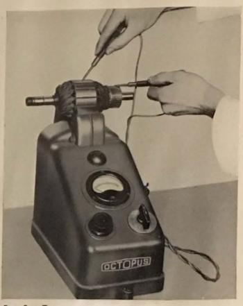
Fig. 9. Testing armature windings or earths using the growler.
