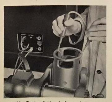
Fig. 12. Testing field coils for earthed windings.
