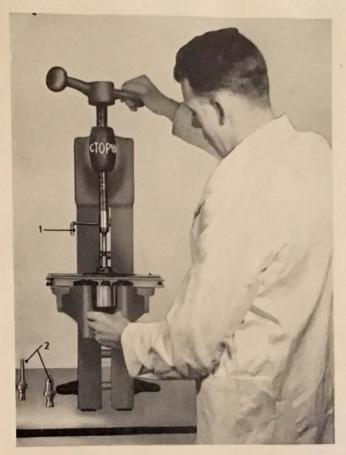
Fig. 3. Using the puller press to remove the end plate from an armature. 1. Tool fixing rod. 2. Tool adaptors.
