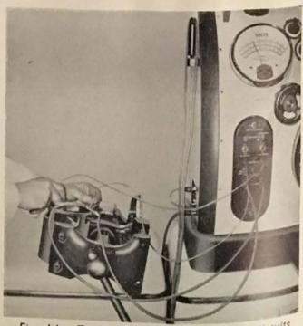
Fig. 14. Testing field coils for short circuits by voltage drop method.
