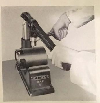
Fig. 4. The pole shoe screwdriver in use.
