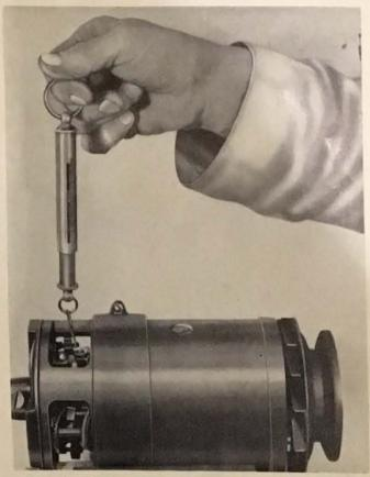
Fig. 7. Testing brush spring tension using spring balance.
