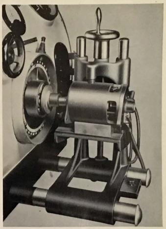
Fig. 15. Generator mounted for test, using hexagon drive coupling.
