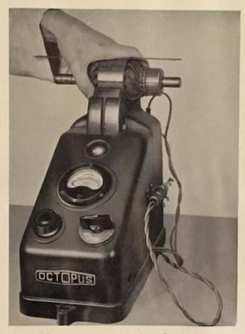
Fig. 10. Testing armature windings for short circuits.
