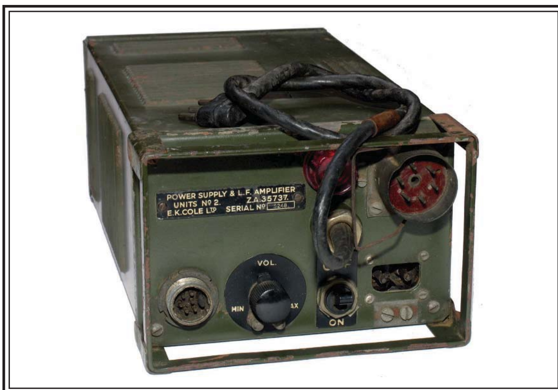
The original 'Power Supply and LF Amplifier Units No. 2', developed for powering a Wireless Set No. 88 AFV in an armoured vehicle and interfacing to the No. 19 Set harness
