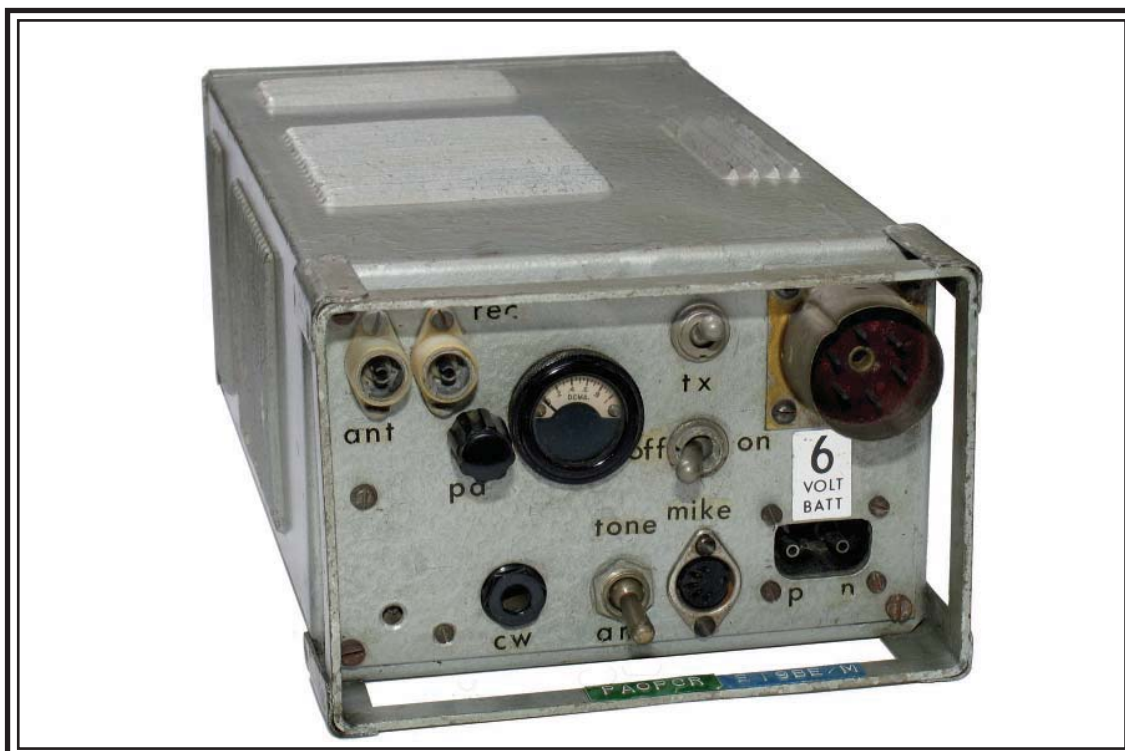
Front panel view of the mobile/portable 2 metre transmitter, a conversion of a war-surplus 'Power Supply & LF Amplifier Units No. 2' described in the Mobile And Portable Operation Of Amateur Radio In The 1960s (Photos by Louis Meulstee)
