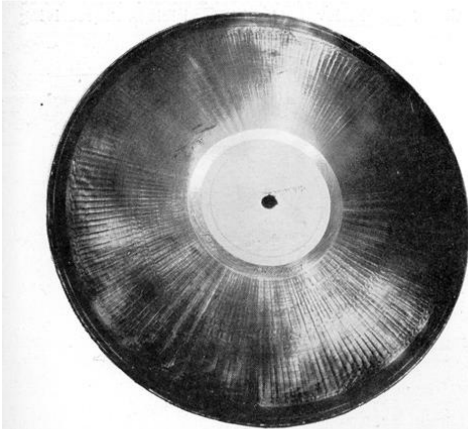
FIG. 85.—An actual phonovision disc record. When “played” on the appropriate apparatus, instead of song or music being heard, the movements of an artist can be watched in the vision apparatus.
