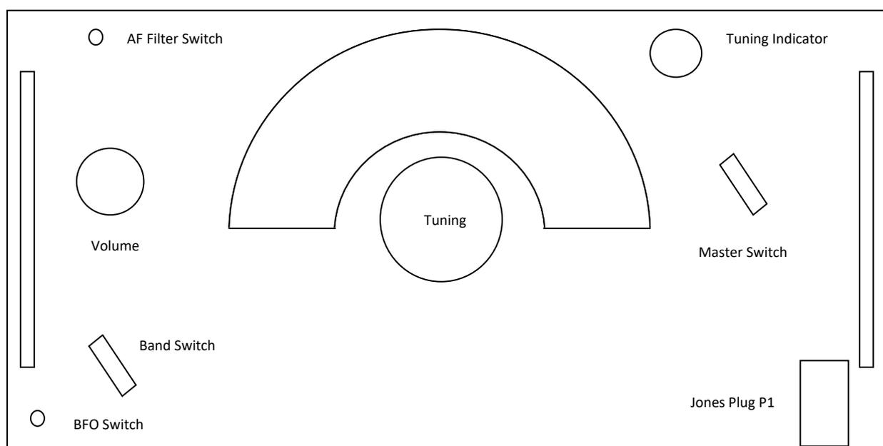
**AF Filter Switch:** In upper position audio is normal. Down position gives bass cut.
