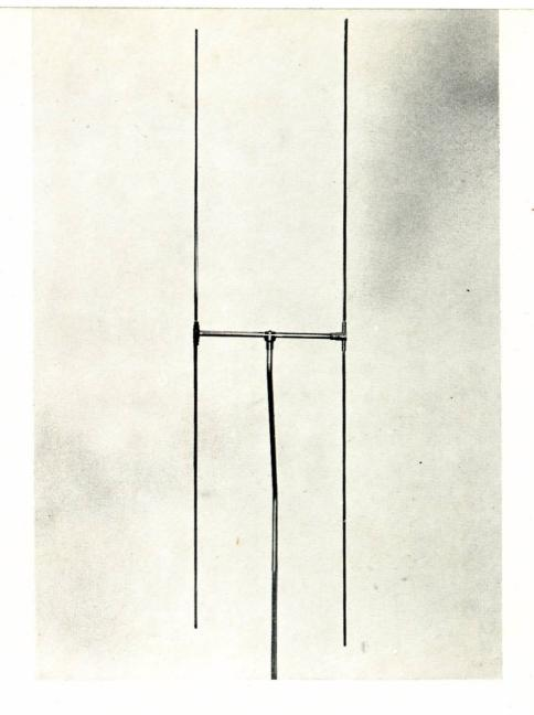
3 DB/CA. \(\frac{1}{8}\) wave spaced H type aerial mounted on cranked arm for chimney fixing. Ideally suited to areas where height is not all-important but where reflections and interference have to be overcome.
